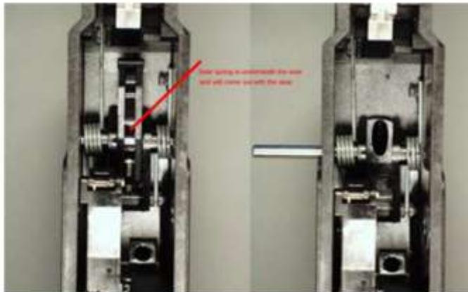
Push the trigger pin half way out.
