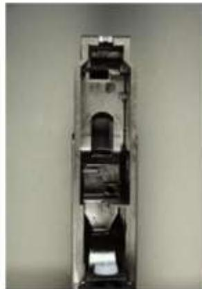
Pull the recessed pin all the way out, releasing the right elbow spring. That's it! You can also remove the white recoil buffer by pulling it straight out with a pair of needle nose pliers.
