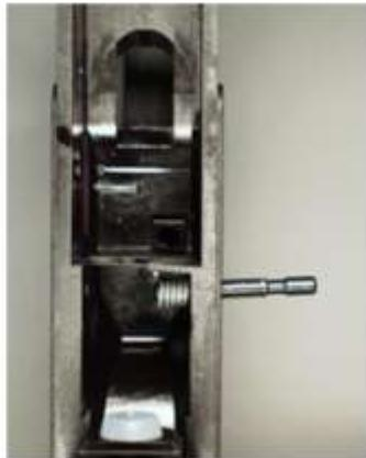
Push the recessed pin half way out to the right. This will allow you to remove the locking lever and the left elbow spring.
