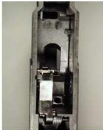
Push the trigger pin completely out and remove the trigger, trigger spring and bolt catch spring. If the locking lever is still in place you'll have to lift it up to get the trigger out.
