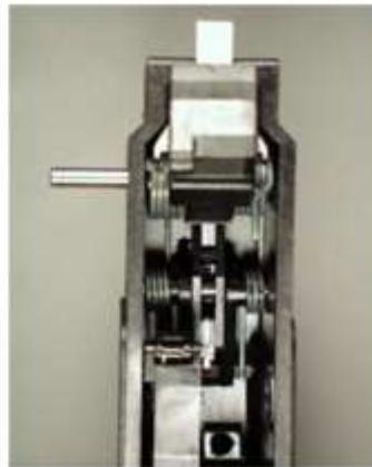
Push out the pin holding the hammer in place. The hammer and hammer springs will now come out.
