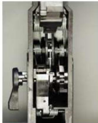
Pull out the left side of the safety lever. You need to lift up the locking lever a bit as you do it.
