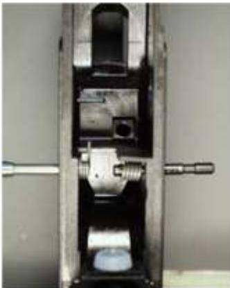
Reassembly is following the same steps in reverse order. One suggestion is to put the trigger back in before the locking lever. Then you won't have to push the locking lever out of the way while working on the trigger.
