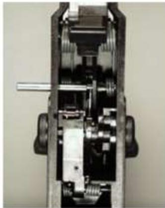
Remove the pin above the trigger.
