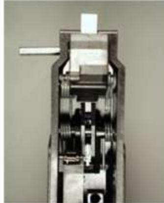
Push out the actuator pin. It's the front most pin in the trigger unit.
