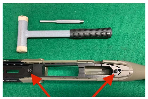
4. Remove the 2 marked screws with a 3mm and 4mm allen key on both sides of the stock.
