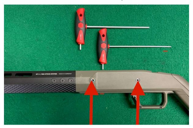
5. Push out the handguard together with the alloy bedding block and remove the 3 marked screws with a 4mm allen key on both sides of the handguard.
