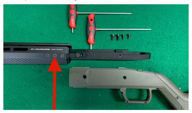
6. Remove the marked screw with a 3mm allen key
